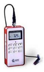
The only way to monitor precisely an individual's exposure to noise is by using either a sound-level meter or a dosimeter. A sound-level meter is a hand-held device that allows a competent third party to take measurements at the operator's ear with the instrument pointing at the noise source. By repeating this exercise for all operations an employee performs during the day, you can calculate his daily exposure.
